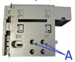
Figure 4 - 12: Removing the Screws
